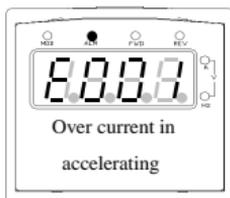
Fig.4-4 failure alarm
