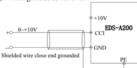
**Fig.3-8 CCI terminal wiring diagram**
