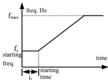
Fig.6-6 Starting freq. and starting time
