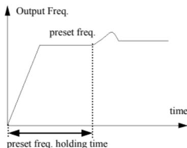
**Fig.6-18 Closed-loop preset freq. run**
