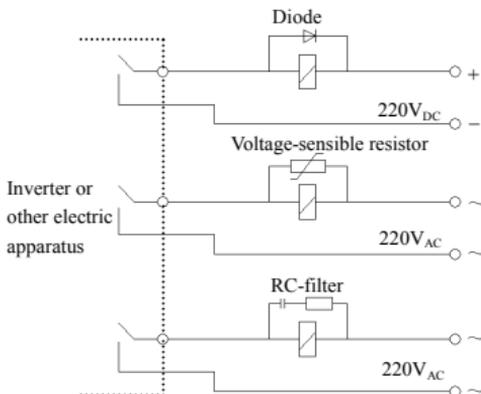
Fig.3-12 Installation demand for electromagnetic on-off device
