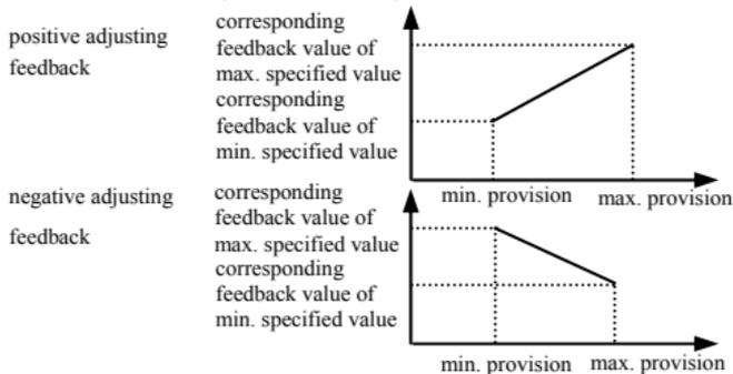
**Fig.6-16 provision, feedback curve**
