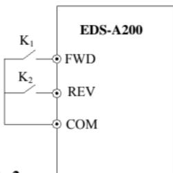
**Fig.6-29 2-wire run mode 2****2: 3-wire control mode 1**
