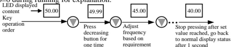
**Fig. 4-8 set frequency adjustment operation example**
