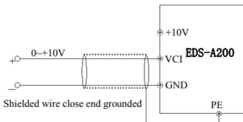
**Fig.3-7 VCI terminal wiring diagram**
