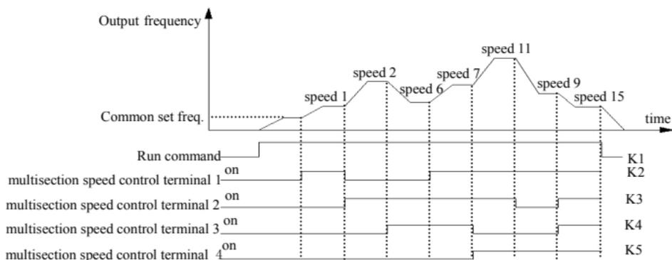
**Fig.6-25 multi-step speed run**
