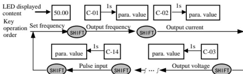
**Fig. 4-6 waiting status parameter display operating example**
