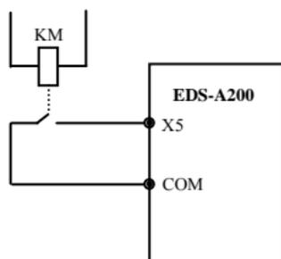
**Fig.6-27 Exterior device failure always-open input**
