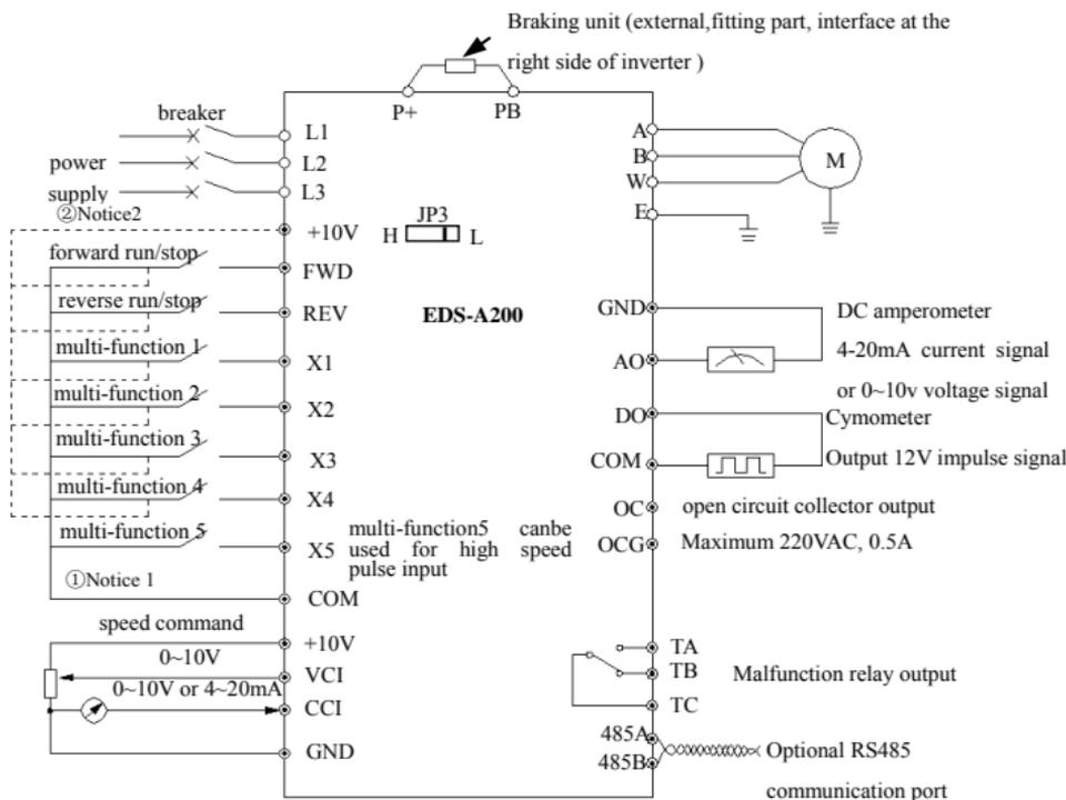
Fig. 3-6 basic wiring diagram
