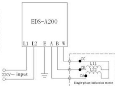
Fig. 3-4 Wiring methods between inverter and motor
