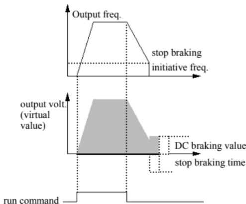
Fig.6-8 Dec stop+DC braking
