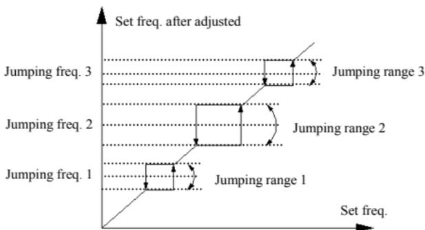
Fig.6-12 jumping frequency and range graph
