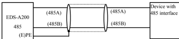
**Fig.3-10 communication terminal wiring**
