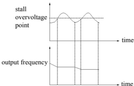
**Fig.6-39 overvoltage stall function**
