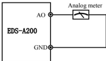
**Fig.3-9 Analog output terminal wiring**
