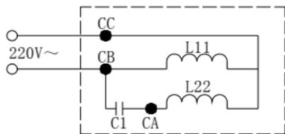
Fig.3-3 Motor inside structure
