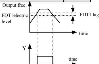
Fig.6-34 freq. level detecting
