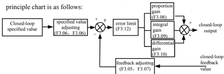
**Fig.6-14 PID control principle diagram**
