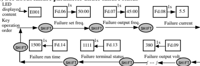
Fig.4-11 Failure status searching operation example
