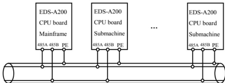
**Fig. 3-11 recommended wiring for multiple inverters communication (all inverters and motors well earthed)**
