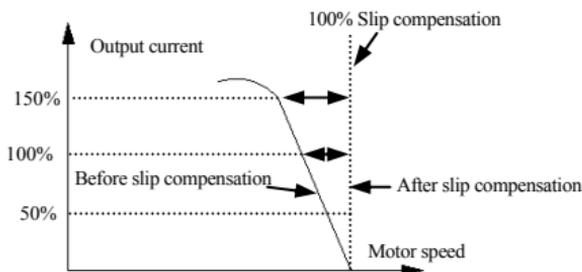
**Fig.6-10 Slip freq. compensation graph**
