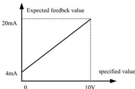
**Fig.6-15 specified value and expected feedback value**
