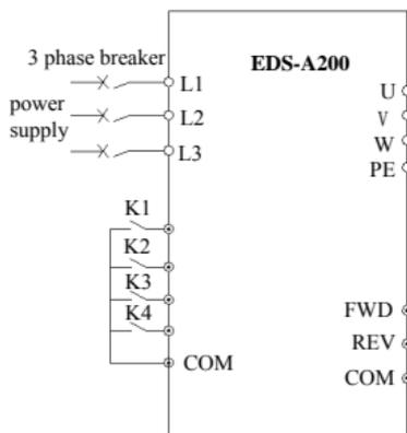
**Fig.6-26 Multi-step speed run**
