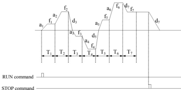
**Fig.6-22 holding mode after PLC single circle**
