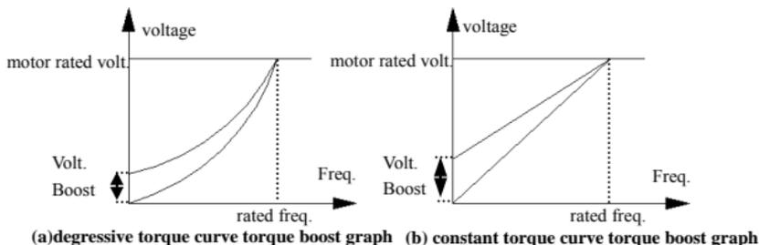
**Fig.6-4 torque boost graph**
