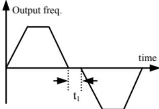
Fig.6-9 FWD REV run dead-section time
