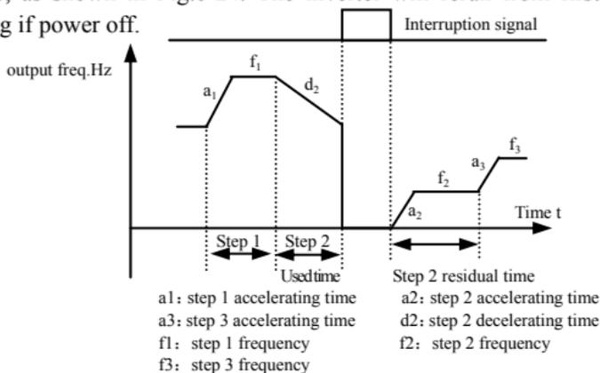
**Fig.6-24 PLC starting mode 1**
